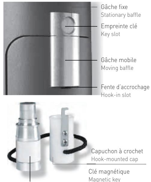
A patented, tamper-proof lock for use on steel pole and column doors (except cylinder and octagonal conical shape). Its opening is triggered exclusively by a special magnetic key. A simple, attractive and durable locking mechanism.
