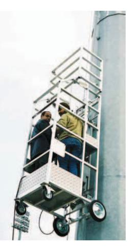
Power lift allow comfortable and secure access to the service platform of large, high lighting masts.
