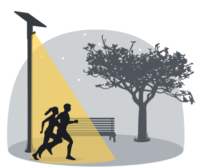
The LED lighting turns on at full power on movement detection.
