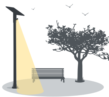
The LED lighting turns on at dusk, when ambient light becomes insufficient.
